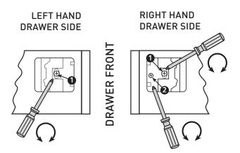
For **Vertical adjustment**, loosen screws **1** adjust Drawer front to desired position, re-tighten screws **1**.
